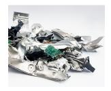
A conventional 3.5 inch hard disk is cut into at least three parts ("H-3 security cut"). The security level is thus many times higher than with conventional methods.
