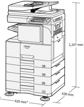
\*Including adjuster. 1,081 mm when finisher tray and multi bypass tray are extended. Show
